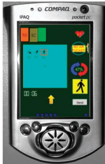
Figure 2.10: The A-Life system shows the victims positions, vital signs and surrounding conditions on a handheld device
