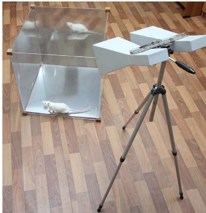
Figure 5. - The experimental set up for estimation of animal's movement activity.
